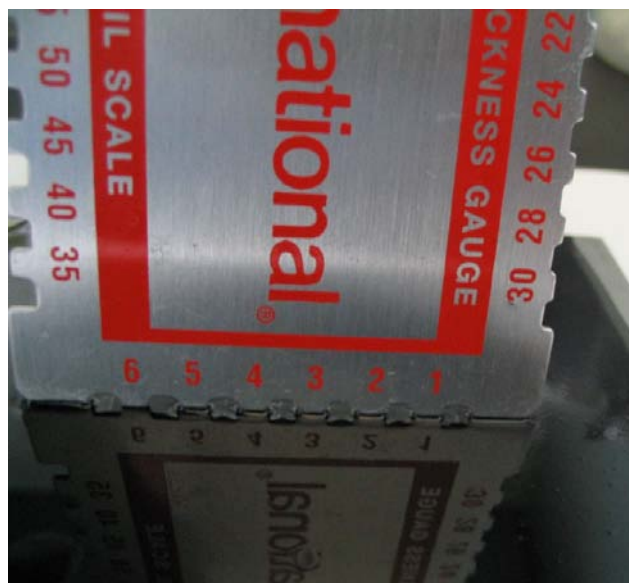
Figure 4. WFT Gauge Positioned in Wet Paint Film.
