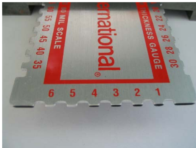
Figure 5. WFT Gauge Showing a Reading of 4-5 Mils.
